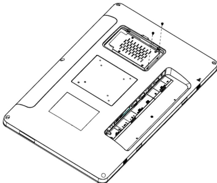
**Step 2.** Insert the HDD back and fasten 2 screws.
