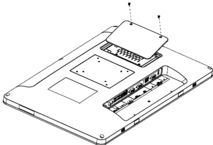
**Step 1.** Remove 2 screws to release the chassis cover, and remove it.
